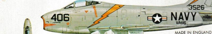
gallon (757 litres) drop tanks. Powered by uprated Wright built J65 Sapphire engine producing 7700 lbs (3493kg) thrust.
