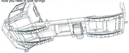
Now you need to build axles. Glue parts together and then cut axles and glue together like on picture. While doing it, measure it with springs. Shorter one is front axle
