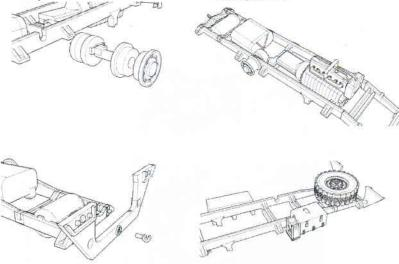
Page 3 Notice, that hook and detailing part for winch (at end) are on end part.
