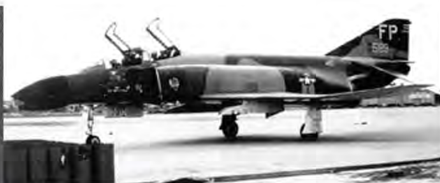
63-7589 taxis in post-mission sometime in late 1967. Note the lack of AIM-9 launcher rails when air-to-ground ordnance was carried
